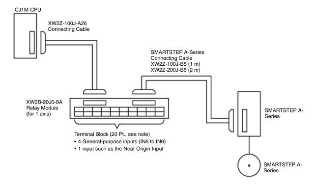
Note: When using a One-axis Relay Module (connected to pulse output 0), general-purpose outputs 2 and 3 (OUT2 and OUT3) and PWM (891) output 1 (OUT5) cannot be used.
